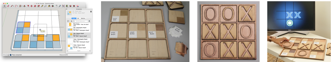
Figure 1. A wireless, batteryless game of Tic-tac-toe is designed using components in the RapID standard library, fabricated using laser cutting along with stick-on RFID tags and foil, and tracked with low latency using the RapID runtime library.
