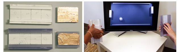
Figure 10. In our pong-like application, two slider components fabricated using different technologies are used to control the paddles in the game.
