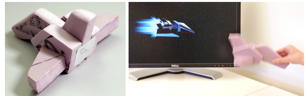
Figure 9. In our spaceship application, a single tag is used to track the motion of a spaceship model. This motion is used to animate an on-screen ship.
