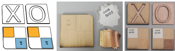
Figure 8. Our Tic-Tac-Toe application’s X and O markers. From left to right: as designed in SketchUp; pending RFID and foil attachment; completed.
