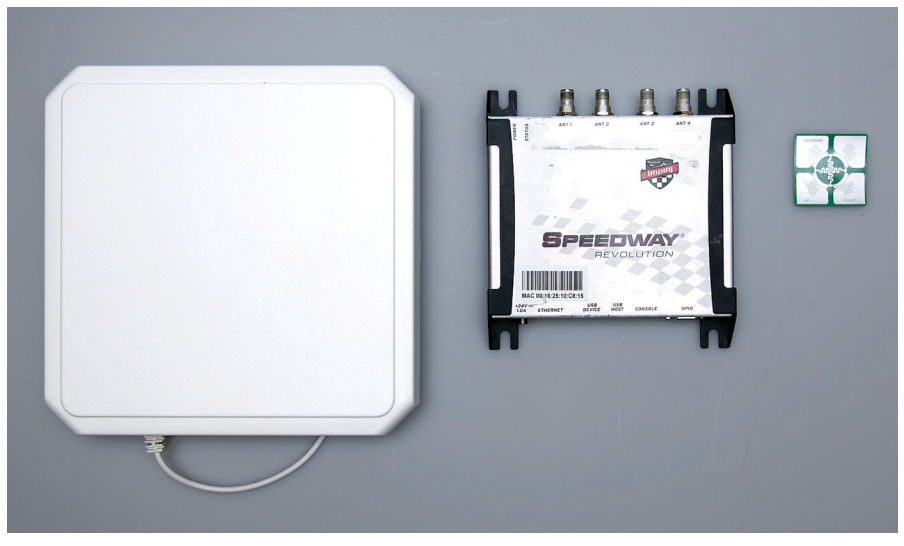
Figure 2: An antenna (left) emits radio waves to a 5.3 cm 2 RFID tag (right), which reflects a response to the reader (center).
