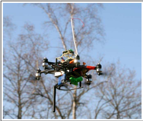
Fig. 2. Our six-rotor helicopter with bird's-eye video camera. The helicopter is 29cm in diameter and weighs 142g without the navigation electronics, camera or communication hardware.
