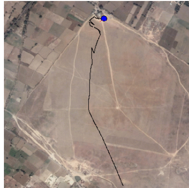
(c) Phase 3 Maximum height: 28.8m Distance traveled: 1290.5m Total flight time: 644.7 sec
