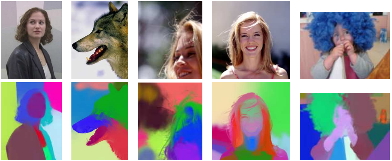
Fig. 4. A number of test images and the matting components extracted from them using our method. A random color is assigned to each component for visualization purposes.
