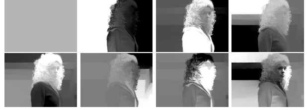
Figure 2. The smallest eigenvectors of the matting Laplacian for the image in figure 1a. Linear combinations of these eigenvectors produced the matting components shown in figure 1d.
