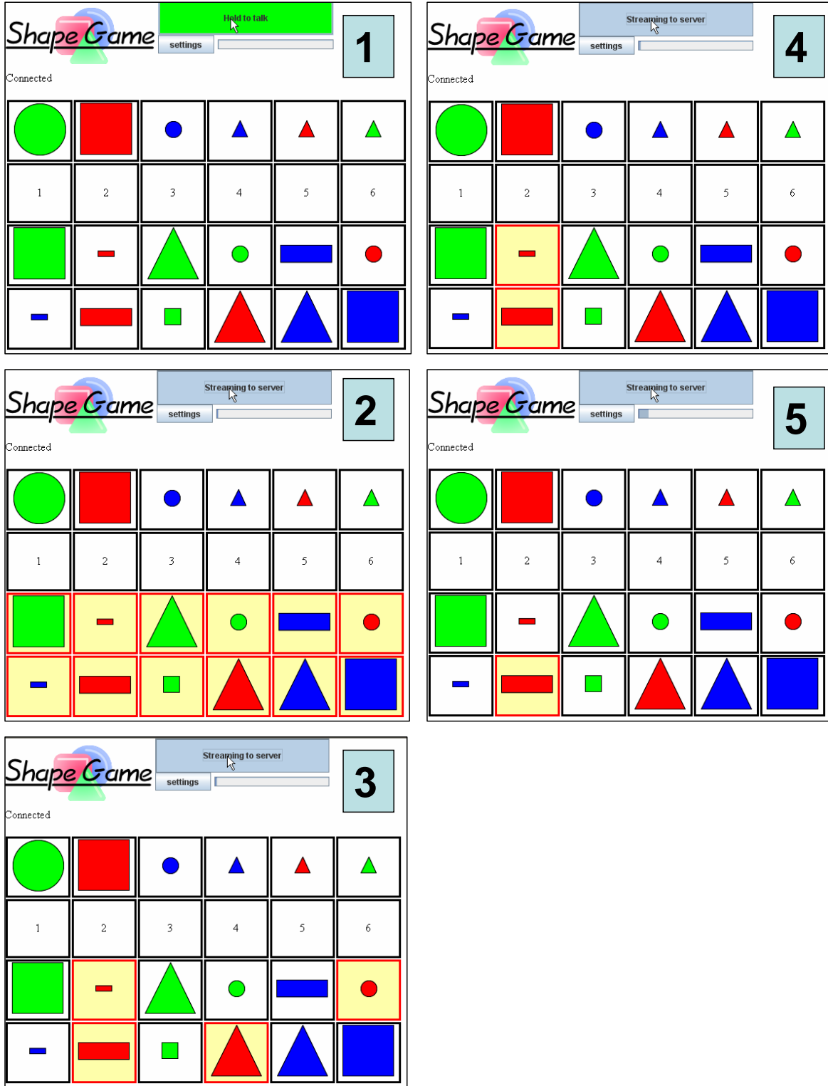
Figure 3: Screenshots of the system as it incrementally responds to a “selection” command: (1) select (2) the red (3) rectangle (4) [pause] the large (5) red rectangle. (Numbers indicate points in the incremental recognition in which each screenshot occurs.) The user gets immediate feedback about which shapes the given constraints select.
