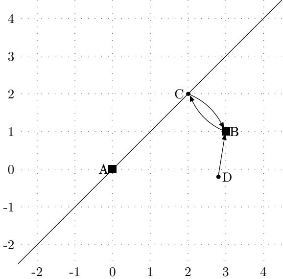
**Fig. 18** An example of a trap resulting from alternating projections. If one alternately projects to the nearest point that satisfies the constraint to be at  $A$  or  $B$ , and then the nearest point where the replica values are equal (the diagonal line), one may be trapped in a short cycle ( $B$  to  $C$  to  $B$  and so on) and never find the true solution at  $A$ .
