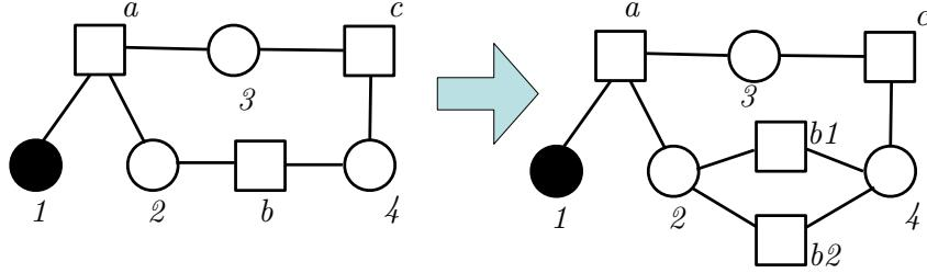
**Fig. 13** One can obtain a new factor graph modeling exactly the same cost function by splitting a factor node into two identical factor nodes, each taking half the cost of the original, and connected to the same variable nodes.
