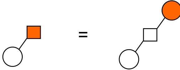
**Fig. 3** Any observed variable nodes in a factor graph can be absorbed as parameters in the factor nodes that they are connected to, leaving only “hidden” variable nodes, and factor nodes that depend on the observations.
