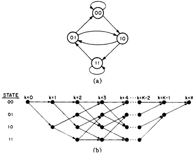
**Fig. 12** An illustration from Forney’s paper [33] on the Viterbi algorithm, showing a state diagram for a four-state shift-register process (a), and the corresponding trellis diagram given evidence for the state of the process from time 0 to time  $k$  (b).
