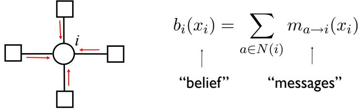
**Fig. 8** The belief update rule for the min-sum BP algorithm says that the belief at a variable node is simply the sum of incoming messages from neighboring factor nodes.
