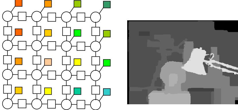
**Fig. 6** An illustration of a factor graph equivalent to a pairwise Markov random field (left) as is often used to representing a computer vision problem, and a depth map returned by a BP algorithm [11] using stereo images (right). The variable nodes in the factor graph could represent unknown depth values, for which there exists some local evidence (the colored factor nodes), and which are statistically correlated (depths at particular pixels tend to be similar to nearby pixels).
