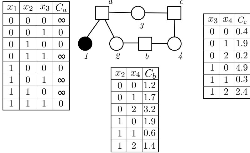
**Fig. 2** A factor graph, along with the lookup tables associated with each local cost function. Note that for this factor graph the four variables are all discrete. Factor  $a$  is a “hard” constraint, that either allows or disallows different local configurations, while factors  $b$  and  $c$  are “soft” factors.
