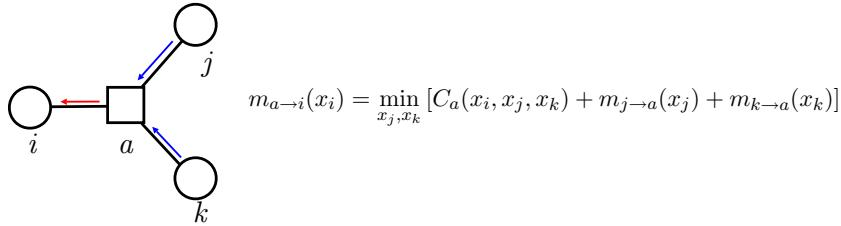
**Fig. 10** The factor-to-variable message update rule for a message from factor  $a$  to variable  $i$  depends on the local cost function  $C_a$ , and the incoming variable-to-factor messages on other edges.
