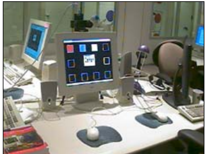
Figure 5: Our experimental setup. Note dual mice, and stereo camera positioned above display screen.
