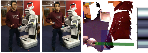
Figure 9: A vertical scan is performed at 2.39 GHz. The estimated location of the concealed object is shown as a green rectangle on the range-image. The loss sequence is shown on the right.
