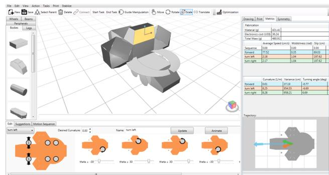
**Figure 3.** User interface. Icons that link to geometry components are displayed on the left and the gait design tool is on the bottom. Users design models by dragging components into the center canvas and editing them. Performance metrics for the design are shown on the right.
