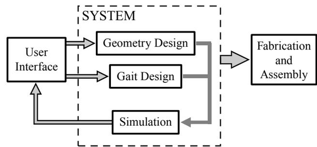
**Figure 2.** System diagram. Users interact with geometry and gait design tools. The designed models are simulated to provide feedback to the user. The user may iterate over the design before fabricating and assembling the model.
