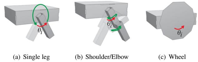
**Figure 8.** Joint controllers for each joint type. Controllers for every joint are separated into a step phase (shown in green) and a reset phase (shown in red). Users modify gaits by changing the  $\theta_i$  values for each joint and defining the step sequence.
