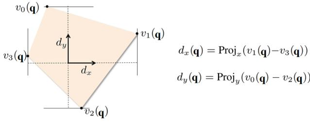
**Figure 6.** Given an orthonormal orientation  $(x, y)$ , the dimension of the part in each direction is written as a function of  $\mathbf{q}$  by using the parametric representation of the extreme vertices.
