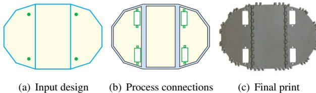
**Figure 12.** Our system automatically generates a 3D mesh for a foldable design. (a) The original design, with blue edges indicating static connections and green dots indicating functional connections. (b) Connections are processed by shrinking faces to make room for hinges and adding holes for servo mounts. (c) Hinges are added and the result is a complete mesh that is 3D printed.
