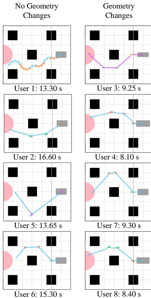
**Figure 15.** Trajectories designed by users during the second task. Users who were allowed to make changes to the robot geometry were able to make the robot navigate the course about 40% faster on average.
