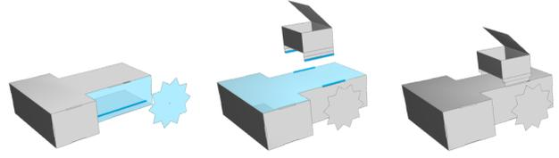
**Figure 7.** As the user drags in components, the UI highlights the patch pairs that will be connected. Limbs are attached to bodies along functional patches. All other components attach via static patches.
