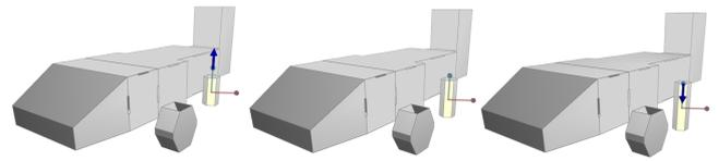
**Figure 10.** The system provides guidance arrows for users who want to make local geometry optimizations. The up and down arrows indicate that the user should lengthen and shorten the leg respectively. No arrow indicates that the part dimension is already at a local optimum.
