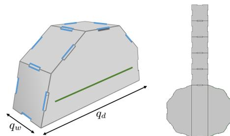
**Figure 5.** One of the geometry components in the database, with both its 3D shape and 2D unfolding. The component has parameter values of diameter  $q_d$  and width  $q_w$ . The green line indicates a functional patch, and the blue lines are static patches.
