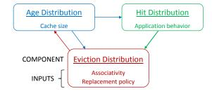
Figure 1: Our model consists of three interdependent probability distributions. Each distribution captures distinct model inputs. Arrows denote dependencies:  $A \rightarrow B$  means "A depends on B".
