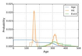
Figure 2: Model solution with increased step size on a synthetic benchmark. Solid lines show a full-detail solution; dashed lines show a solution with N = 32.
