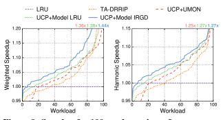
Figure 9: Speedup for 100 random mixes of SPEC CPU2006 apps. Our model enables partitioning of IRGD, improving performance over the state-of-the-art.
