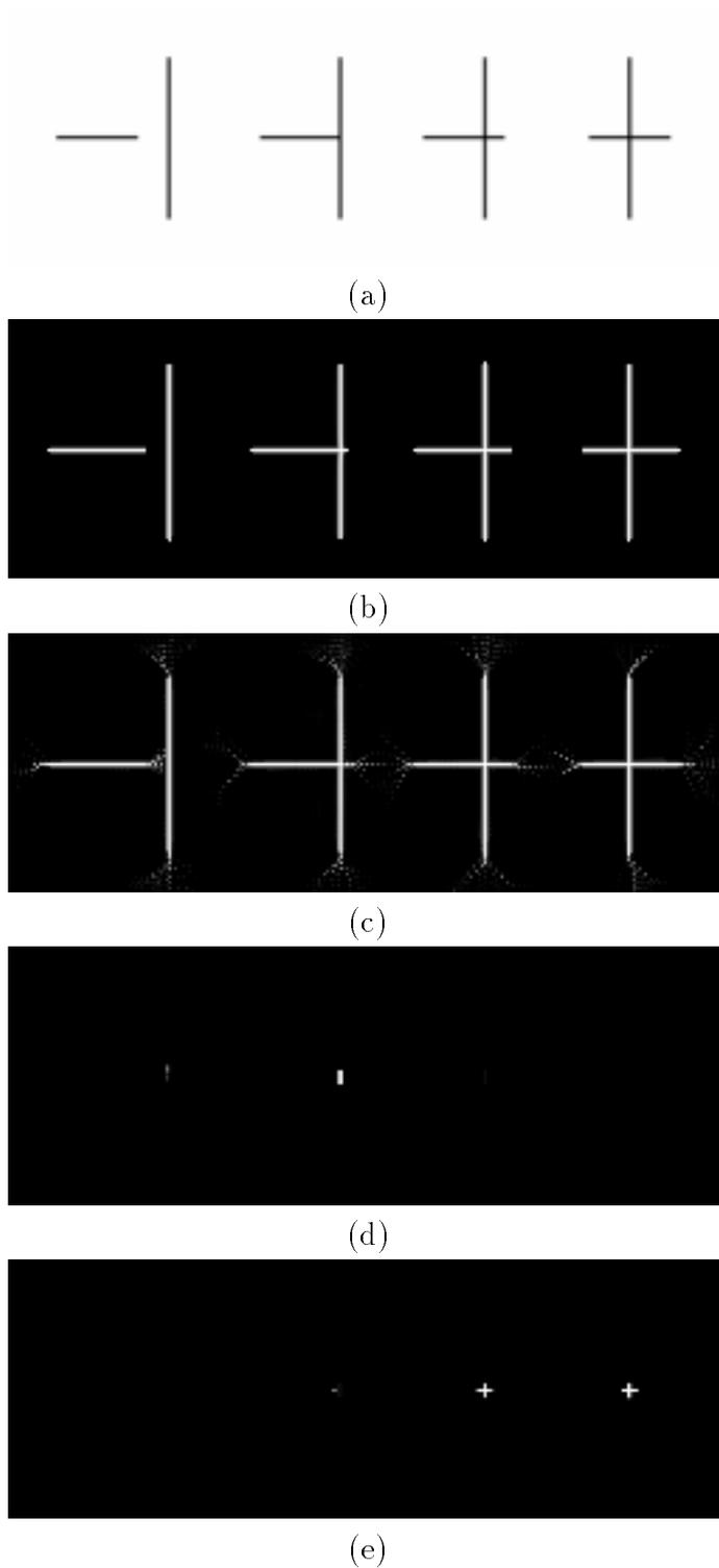
**Figure 6-10:** Showing system response to junctions which show a gradual change in type from T to X. (a) Image. (b) Contour data input to cooperative network. (c) Maximum over all orientations of modified saliency. (d) and (e) show the local evidence for occlusion and transparency, respectively. Note the smooth transition from T-ness to X-ness.
