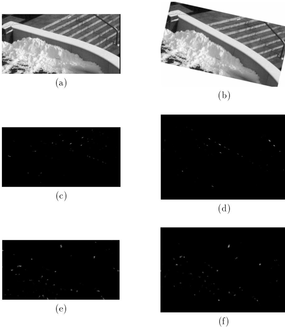
**Figure 6-19:** Orientation dependent results, continued from Fig. 6-18. Input images (a) and (b) are repeated, for convenience. The orientation dependence of the saliency outputs affects the junction analysis, as shown by the different outputs of the T-junction detectors, (c) and (d). For comparison, the outputs of the energy based T-junction detector of Chapter 5 are shown in (e) and (f). These T-junction measurements are substantially invariant to rotations.
