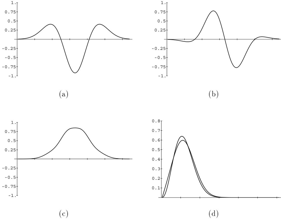
**Figure 2-4:** (a)  $G_2$ , 2nd derivative of Gaussian (in 1 dimension). (b)  $H_2$ , fit of 3rd order polynomial (times Gaussian) to the Hilbert transform of (a). (c) energy measure:  $(G_2)^2 + (H_2)^2$ . (d) magnitudes of Fourier transforms of (a) and (b).
