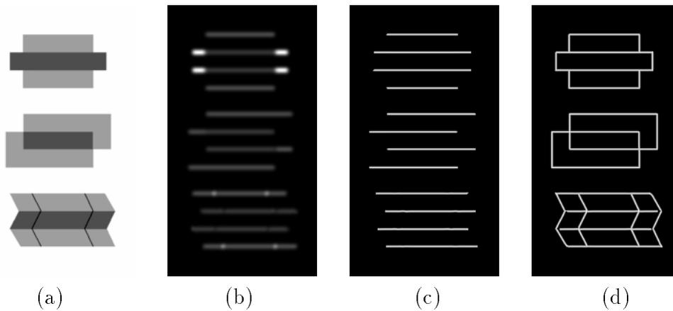
**Figure 6-4:** From image to oriented contours. (a) Test image. (b) blurred horizontal oriented energy. Note high dynamic range because of the range of image contrasts. (c) Horizontal contour strength, calculated as described in text. (d) Union of contours found for all orientations.
