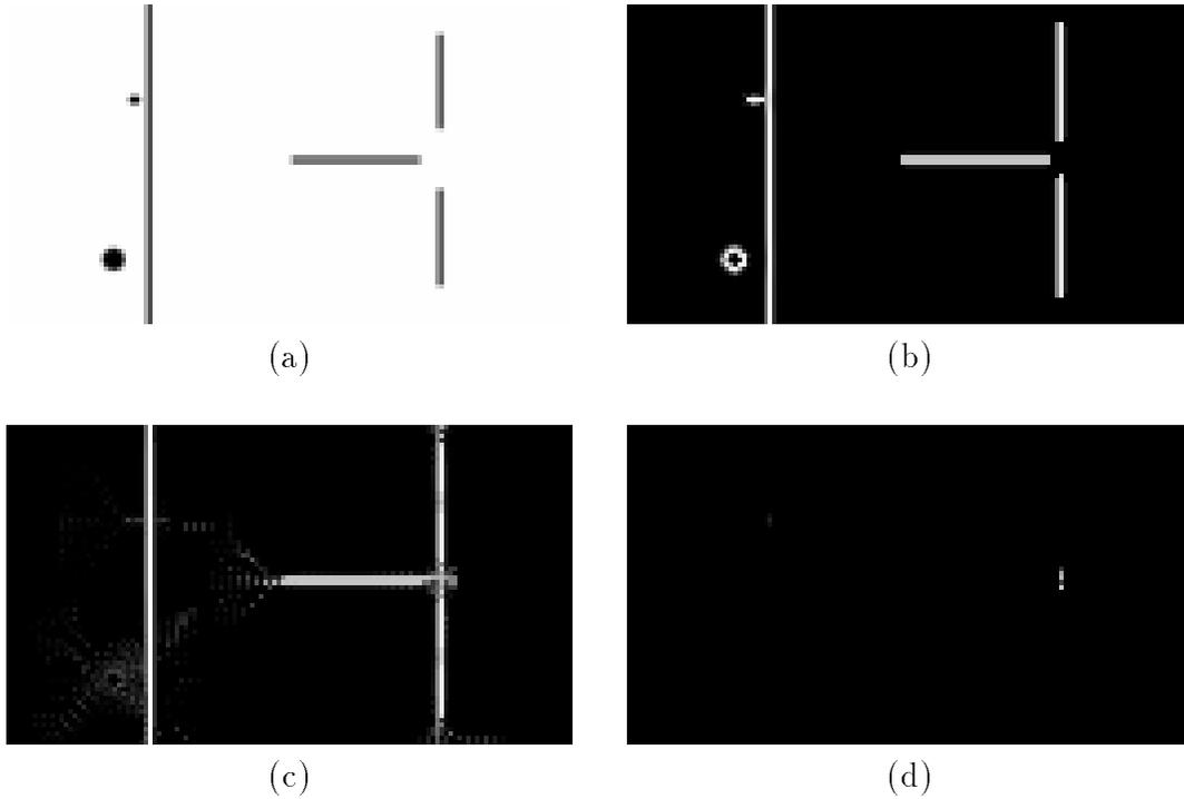
**Figure 6-11:** Images showing the advantages for junction detection of an approach based on salient contours. (a) Image for which the methods of Chapter 5 fail. (b) Contour data input to cooperative network. (c) Maximum over all orientations of the output of the cooperative network, the modified saliency. (d) shows the local evidence for occlusion. The T-junction detector correctly finds no T-ness in the left figure but does respond to the other figure, despite the gap.
