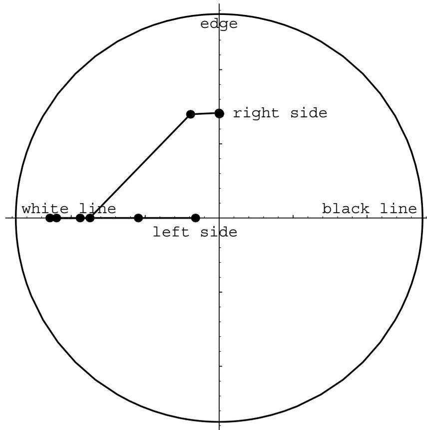
**Figure 4-8:** Polar plot of the energy and phase at positions of energy local maxima for the test image of Fig. 4-7. The data points corresponding to the far right and left sides of the test image are labeled. There are actually 19 data points superimposed on the exact same dot at edge phase (“right side”), illustrating the bias toward strong edges in the simple image model of Fig. 4-7. This bias is observed in real images.
