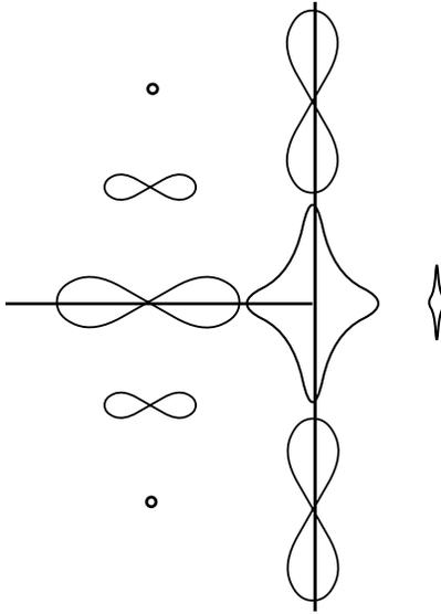
**Figure 5-5:** Local energy measures can be used to identify T-junctions. Floret polar plots of oriented energy as a function of orientation are shown for various positions near a T-junction. This plot illustrates the local energy characteristics which we require for a T-junction: the energy perpendicular to the two dominant orientations must be at a local maximum; and the energy along the dominant orientations must show end-stopping for exactly one of the two orientations.
