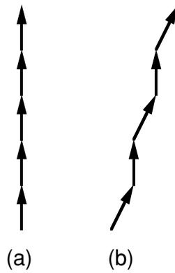
**Figure 6-17:** Illustrating saliency artifact due to quantization in orientation. The saliency of a straight line should be independent of its orientation. However, a line parallel with one of the orientation axes, as in (a), will have unity coupling constant between links, while one between two orientation axes could have a weaker coupling constant for every link. This worst case is analyzed in the text.
