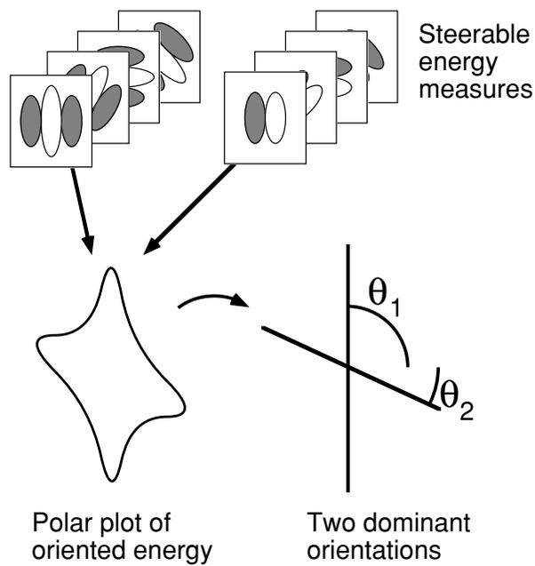
**Figure 5-6:** Initial processing in junction detection. A bank of steerable quadrature pair filters measures oriented energy as a function of angle. The two dominant orientations are defined to be the angles corresponding to the two strongest energy local maxima.
