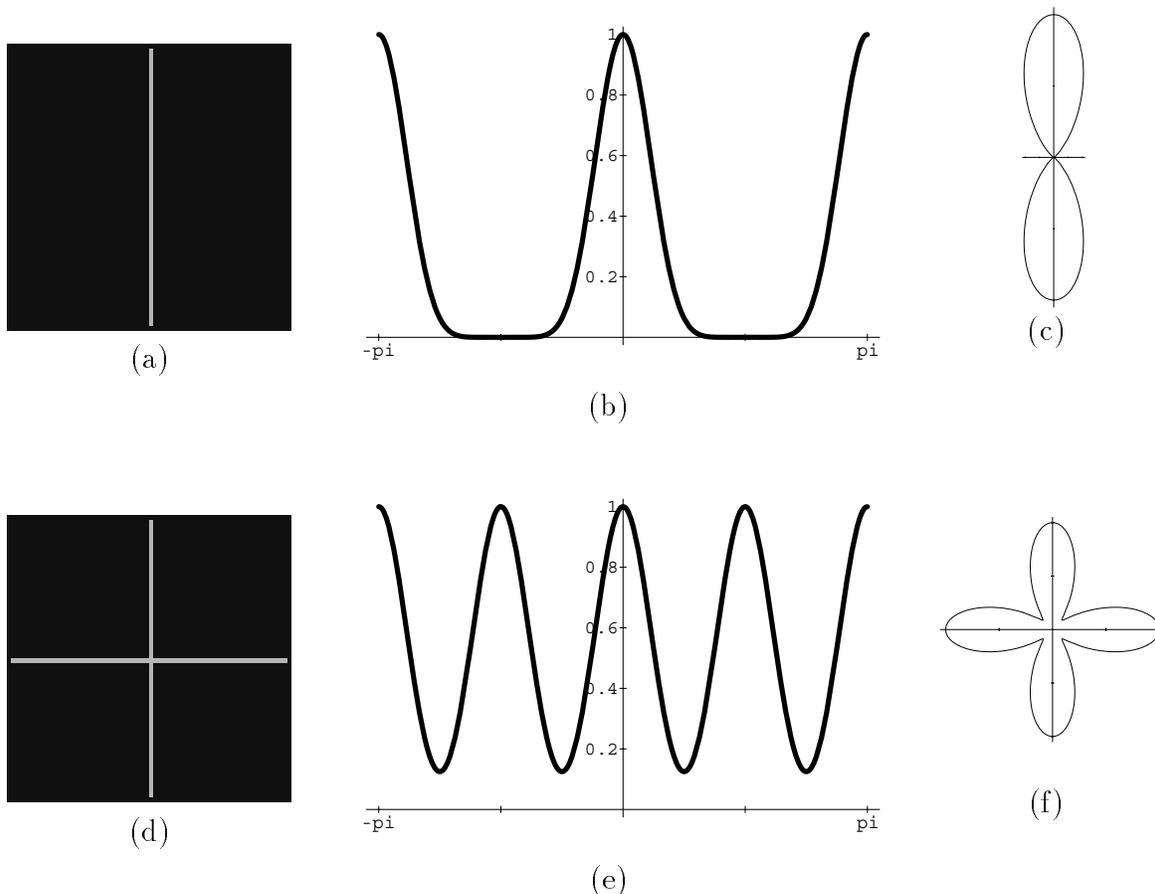
**Figure 3-2:** Test images of (a) vertical line and (b) intersecting lines. (c) and (d): Oriented energy as a function of angle at the centers of test images (a) and (b). Oriented energy was measured using the  $G_4$ ,  $H_4$  quadrature steerable pair. (e) and (f): polar plots of (c) and (d).
