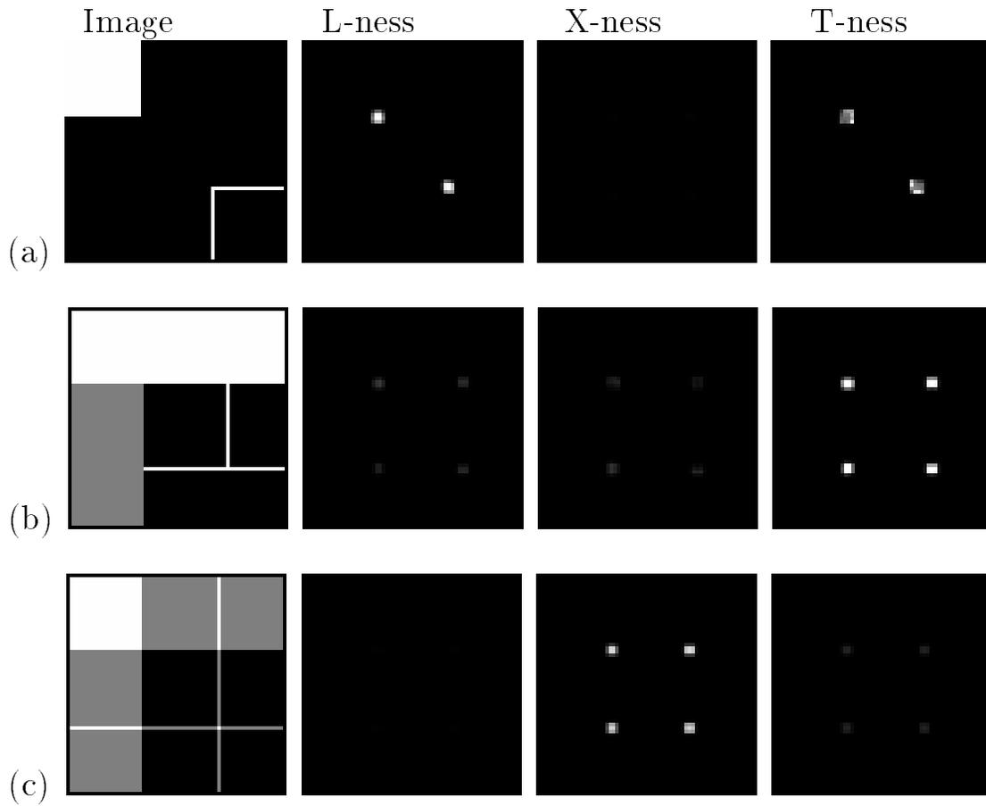
**Figure 5-11:** Showing outputs of local junction detectors made from oriented filter outputs. Test images are composed of (a) L-junctions, (b) T-junctions, and (c) X-junctions. In each case, the correct filter responds at the desired location, and the incorrect filters do not respond significantly. Note that the detectors operate correctly on junctions composed of either lines or edges.
