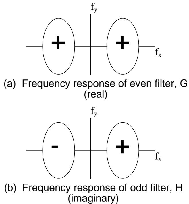
**Figure 3-5:** Frequency content of two bandpass filters in quadrature. (a) even phase filter, called  $G$  in text, and (b) odd phase filter,  $H$ . Plus and minus sign illustrate relative sign of regions in the frequency domain. See Fig. 3-6 for calculation of the frequency content of the energy measure derived from these two filters.
