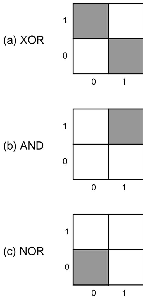
**Figure 6-8:** Intuition behind the junction classification scheme of Fig. 6-9. The (a) XOR, (b) AND, and (c) NOR functions correspond to the classifications for evidence for T-junctions, X-junctions, and no junction, respectively, in Fig. 6-9.
