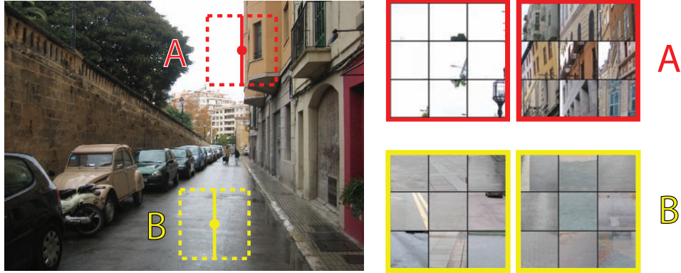
Figure 2: Data driven boundary detection. Left: Input image with query edges shown. Right: The top 9 matches in a large collection of images for each side of the query edges. Rank correlation for occlusion boundary (A): -0.0998 ; rank correlation within the road region (B): 0.6067 . Notice that for point B lying inside an object (the road), the ranked sets of retrieved images for the two sides of the oriented line are similar, resulting in a high rank correlation score. At point A lying at an occlusion boundary between the building and the sky, the sets of retrieved images are very different, resulting in a low rank correlation score.
