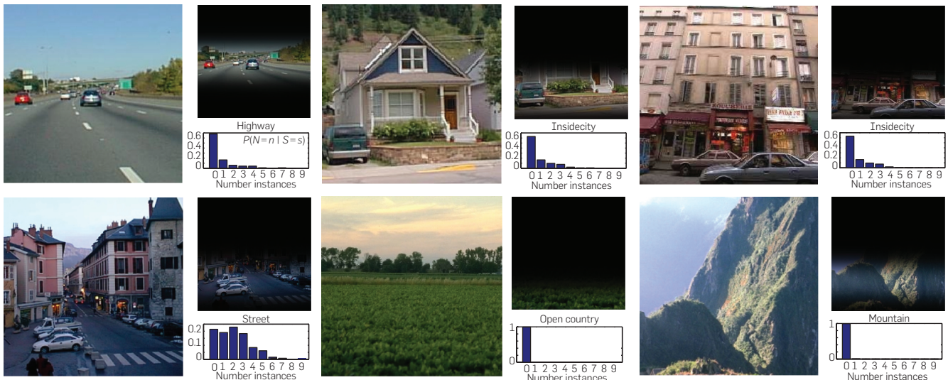
Figure 4. Predicting the presence/absence of cars in images and their locations using gist. The outputs shown here do not incorporate any information coming from a car detector and are only based on context. Note that in the dataset used to fit the distributions of object counts for each scene category, it is more common to find cars in street scenes (with many cars circulating and parked) than in highway scenes, where there are many shots of empty roads. Hence the histogram for highway shows p(N^{car} = 0) = 0.6 .
