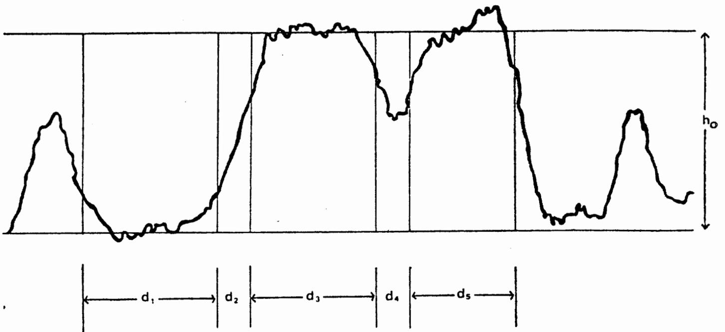
Illustration of the waveform and some of the measurements taken to verify a hypothesized edge position.
