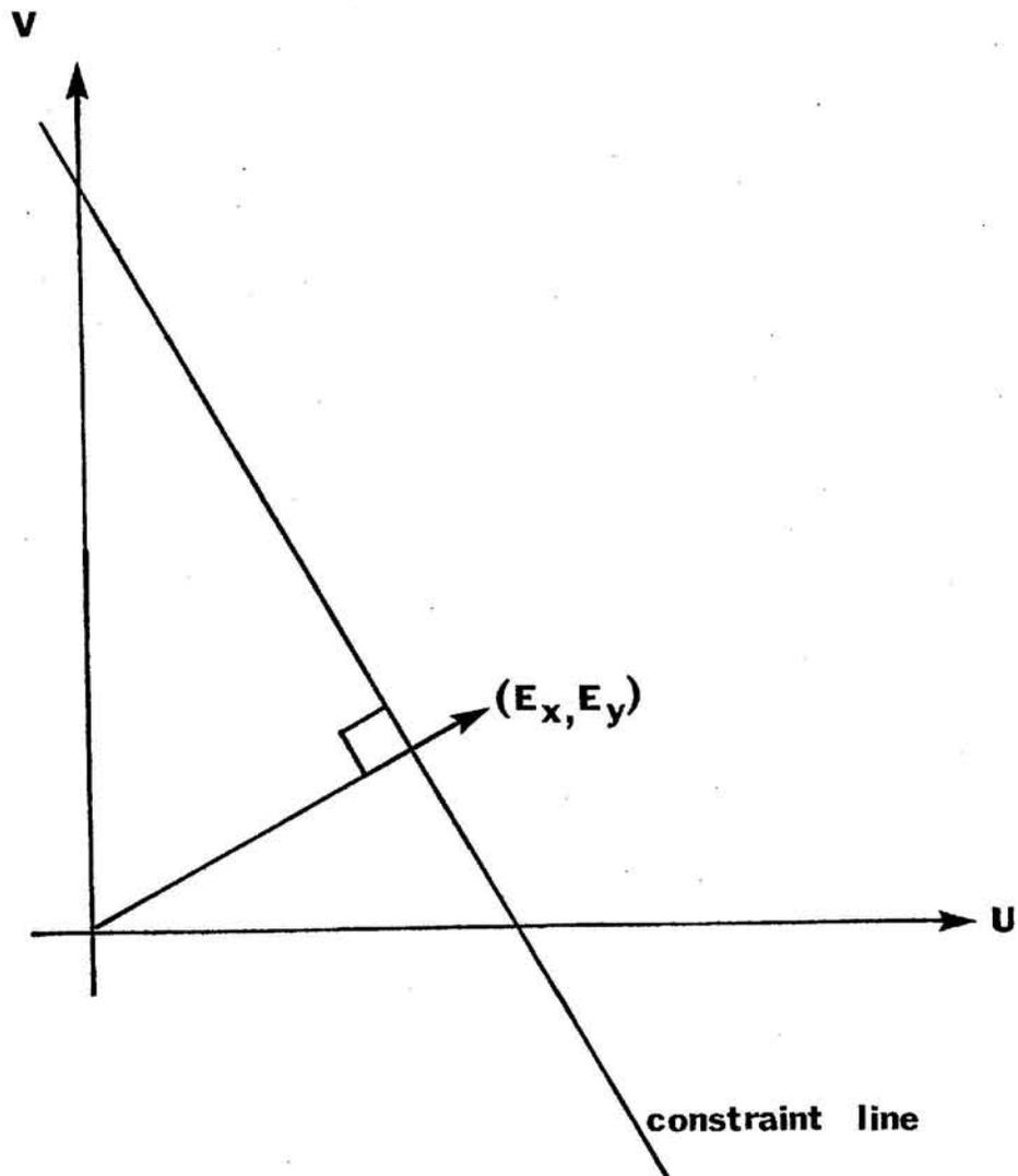
Figure 1. The basic rate of change of image brightness equation constrains the optical flow velocity. The velocity  $(u, v)$  has to lie along a certain line perpendicular to the brightness gradient vector  $(E_x, E_y)$  in velocity space.
