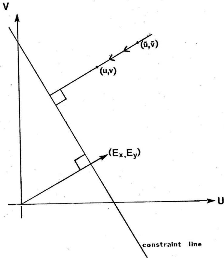
Figure 4. The value of the flow velocity which minimizes the error lies on a line drawn from the local average of the flow velocity perpendicular to the constraint line.
