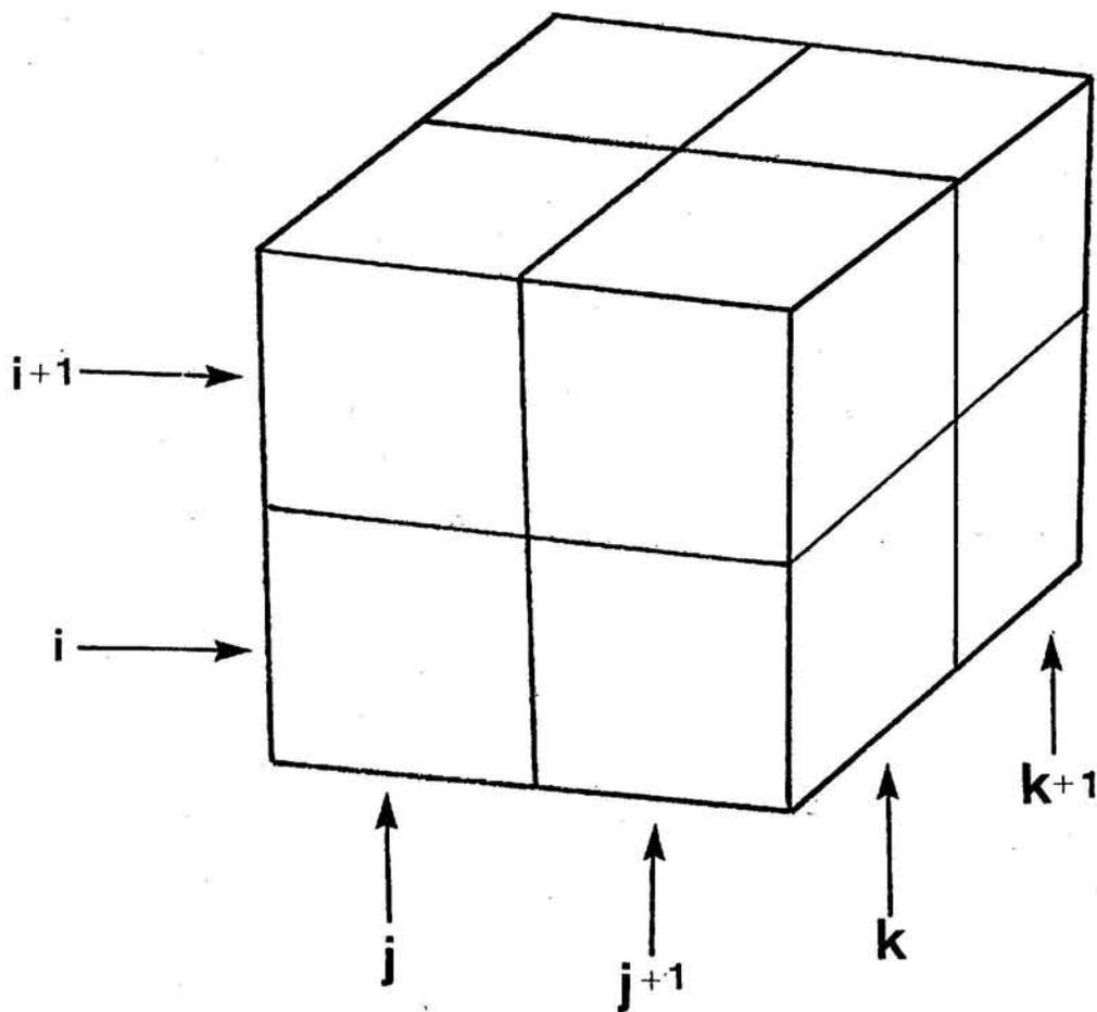
Figure 2. The three partial derivatives of image brightness at the center of the cube are each estimated from the average of first differences along four parallel edges of the cube. Here the column index  $j$  corresponds to the  $x$  direction in the image, the row index  $i$  to the  $y$  direction, while  $k$  lies in the time direction.
