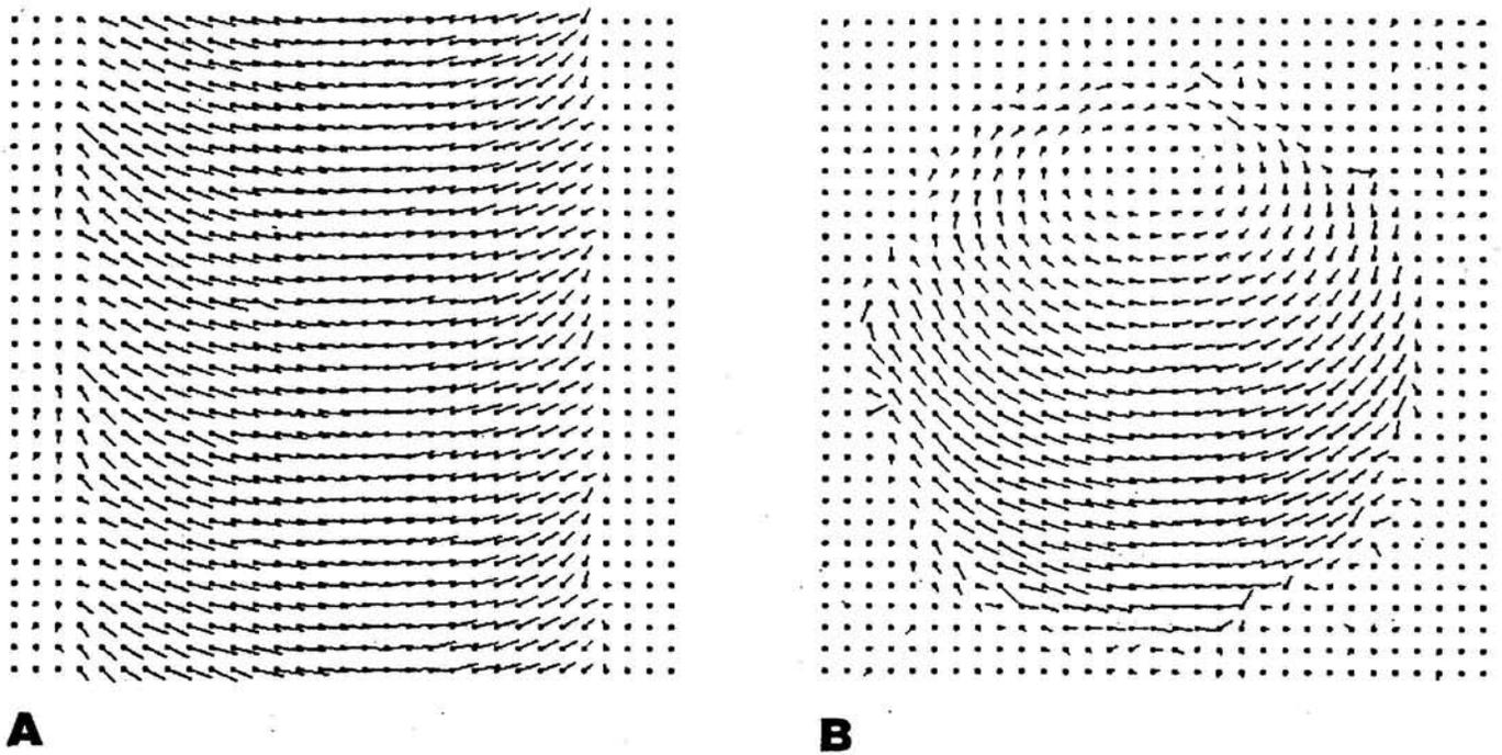
Figure 10. Flow patterns computed for a cylinder rotating about its axis and for a rotating sphere. The axis of the cylinder is inclined 30 degrees towards the viewer and that of the sphere 45 degrees. Both are rotating at about 5 degrees per time step. The estimates shown are obtained after 32 time steps.
