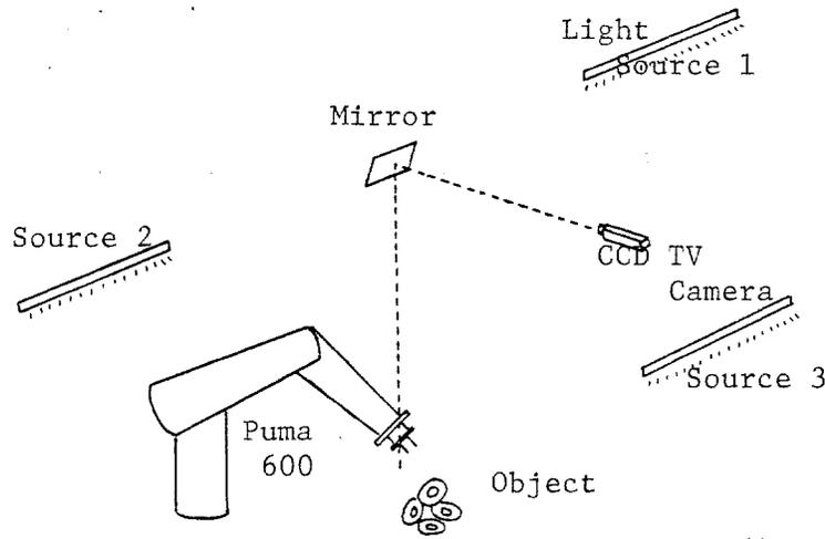
Figure 1. The experimental set up. A CCD camera is mounted in the ceiling and observes the scene through a mirror. Three light sources are controlled by the lisp machine.
