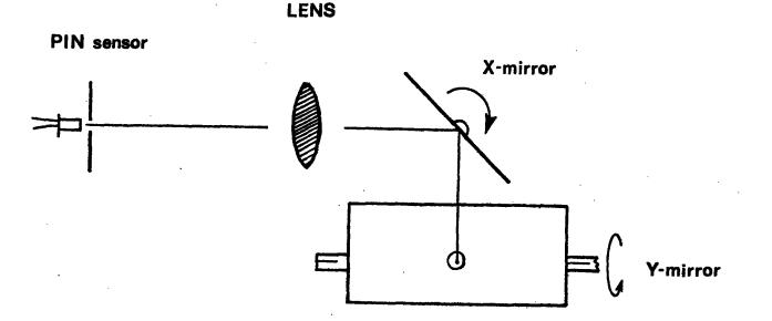
The photo-diode is mounted behind an aperture on the optical axis in the image place of the lens. The lens is aimed at the square x-mirror, which
