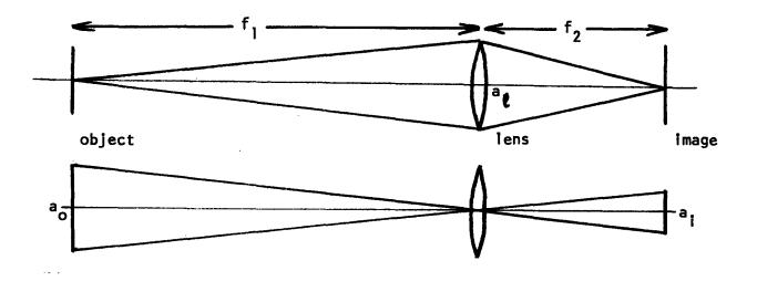
Let the lens have a diameter d and hence an area  $a_1 = (\pi/4)d^2$ . Let the aperture have a diameter e and hence an area  $a_1 = (\pi/4)e^2$ . Let the corresponding piece of the object have area  $a_0 = a_1(f_1/f_2)^2 *$ Then the solid angle per picture cell is  $a_1/f_2^2 = a_0/f_1^2$ .
