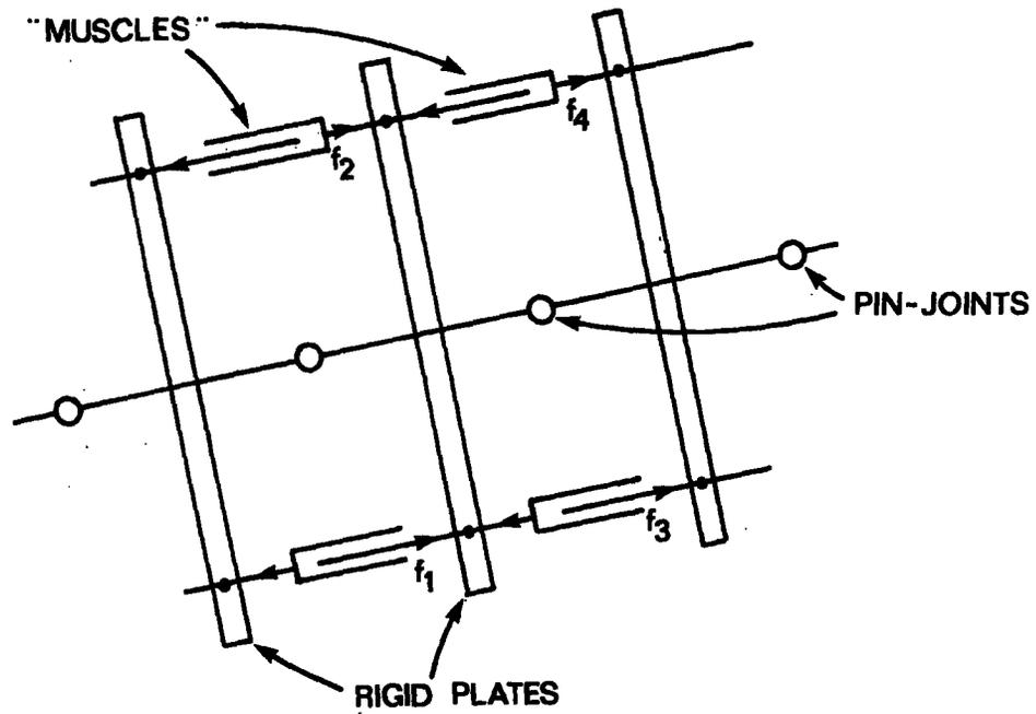
FIGURE 5. Discrete Model of Body Section. The "muscles" generate torques around the pin-jointed "spine". The rigid plates are  $2r$  long and the separation between successive pin-joints is  $\delta$ .
