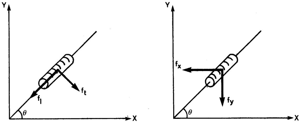
FIGURE 4. Determination of forces per unit length in direction of coordinate axes.
