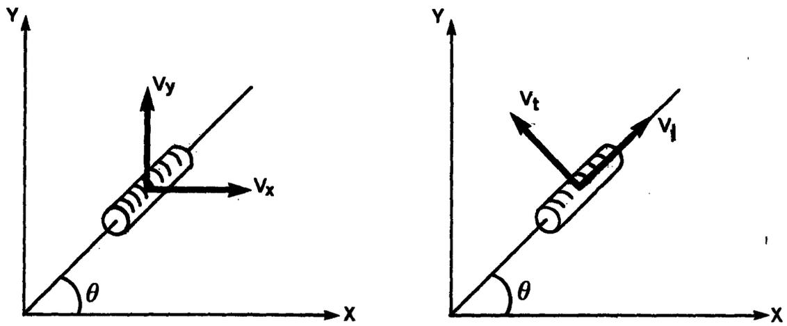
FIGURE 3. Determination of velocity along direction of body segment and velocity at right angles to body segment.
