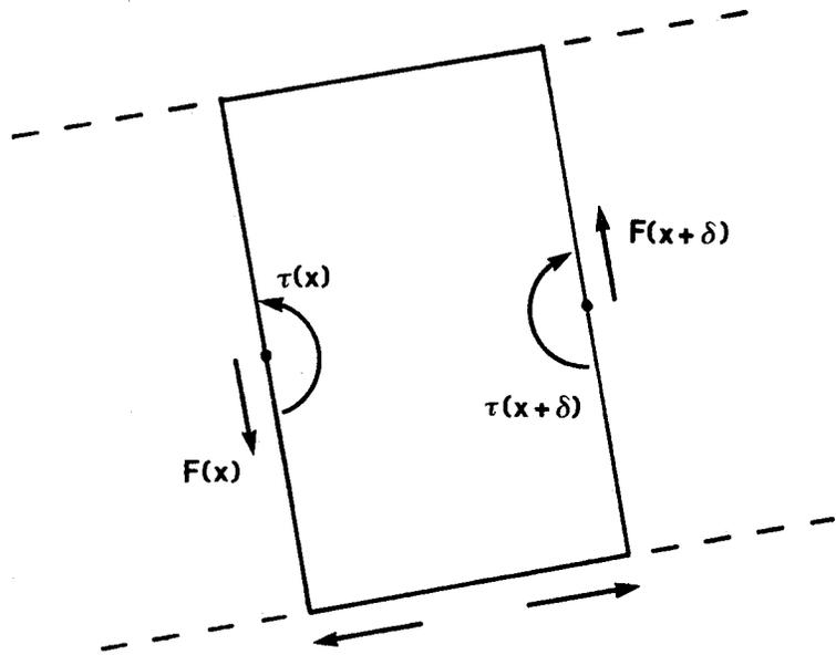
FIGURE 6. Slice of Continuous Model of Body.  $F$  is the shear force across the body, while  $\tau$  is the torque.
