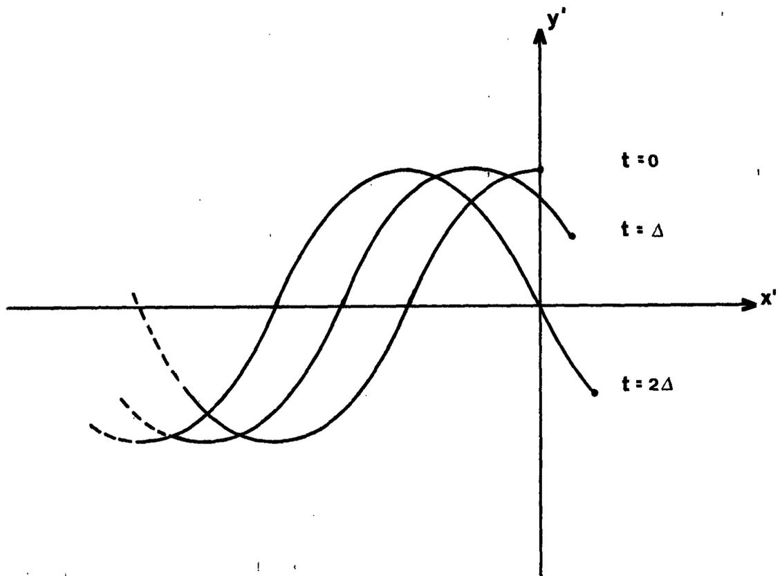
FIGURE 1. Travelling wave of body motion. The amplitude of the wave is  $Y$ , the length of the body is  $L$ . The wave, of angular frequency  $\omega$ , travels backward along the body at velocity  $u$ , while the body is propelled forward at velocity  $v$  relative to the fluid.  $u$  is somewhat larger than  $v$ .
