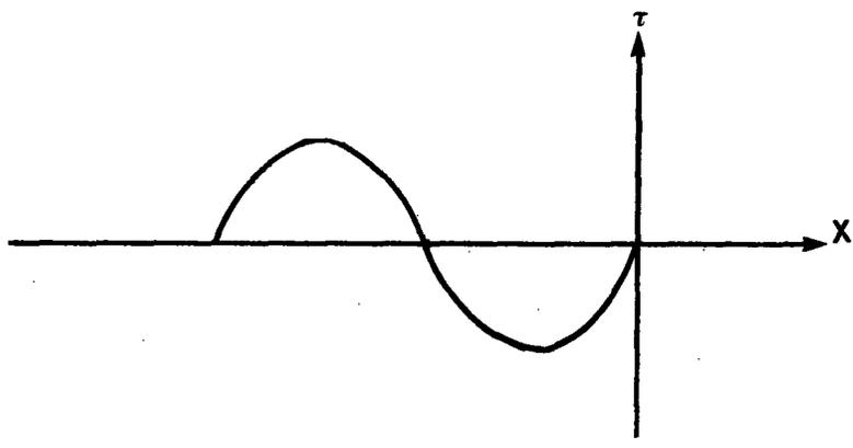
FIGURE 7. Phase relationship between driving torque and displacement for the massless body model.
