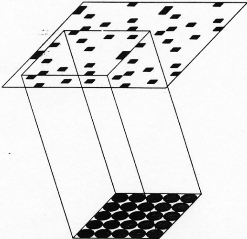
Fig. 1. Diagram of coded aperture imaging system with modular detector. A shadowgram from any one source is only partially sampled.
