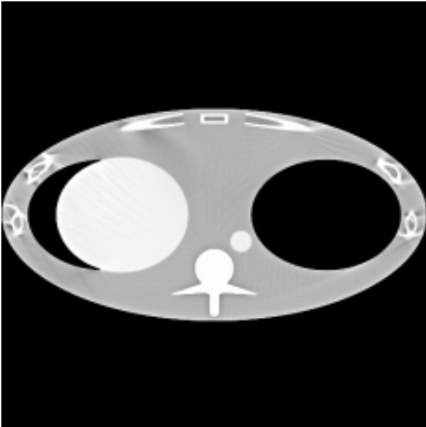
Fig. 4. Axial image of a thorax phantom at pitch 80, reconstructed with AMPR. The field of view is 400 mm; the display window is 200 HU; same slice location as figure 3. Severe artifacts are visible, particularly near the ribs.
