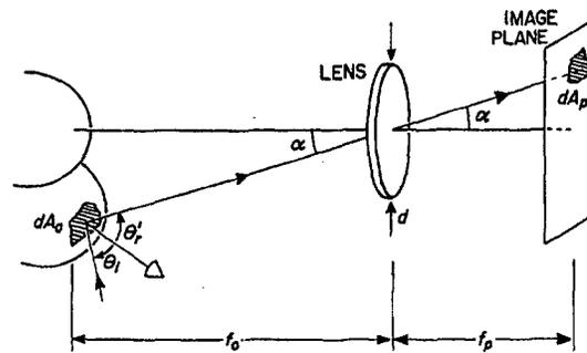
Fig. 8. A simple image-forming system. Light collected by the lens from the surface patch of area  $dA_0$  is projected into the image patch of area  $dA_p$ .
