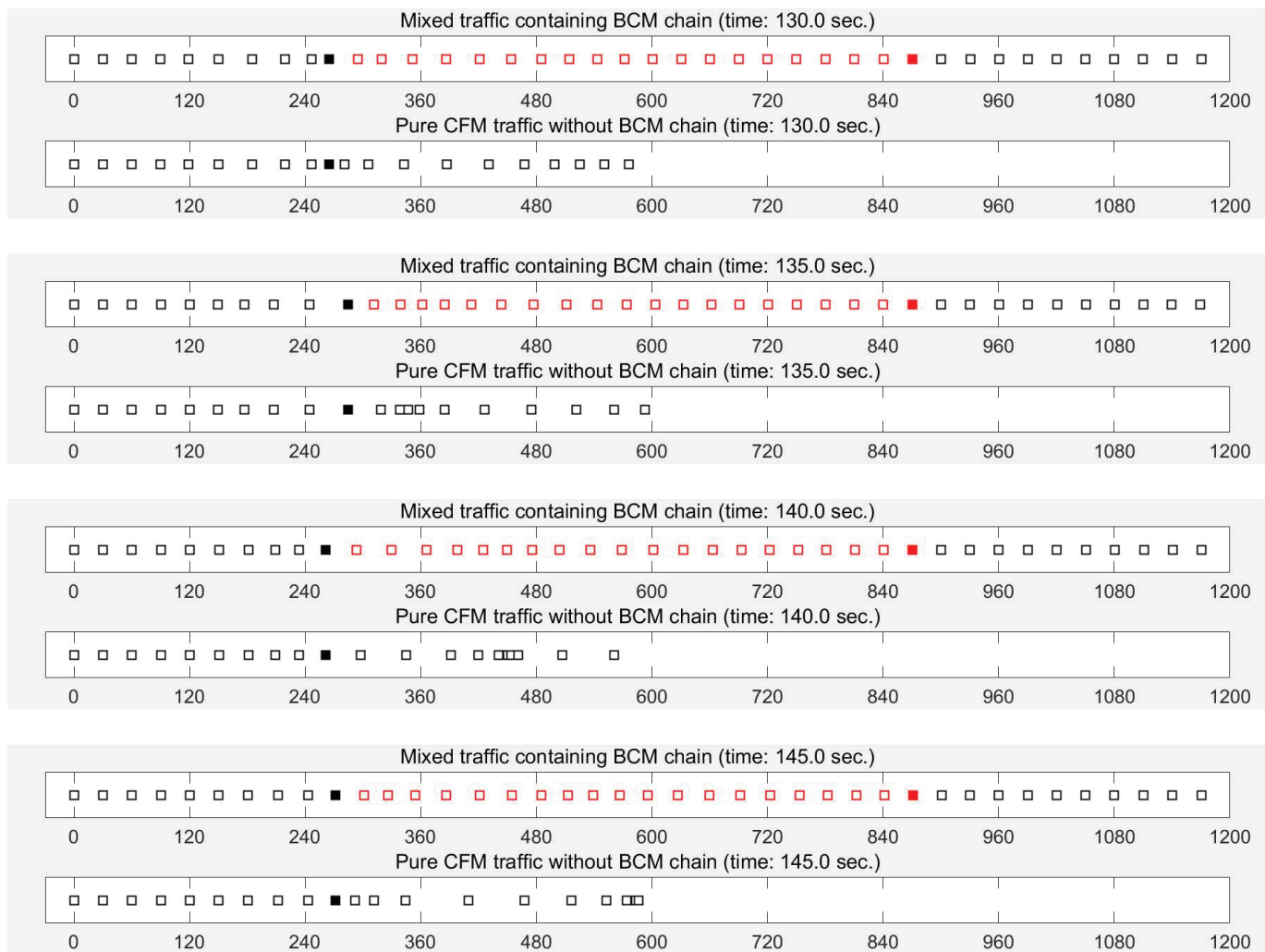
Fig. 9. Some of the simulations results. The black squares indicate the CFM vehicles, while the red squares indicate the BCM vehicles. The solid black square indicates the last car in the CFM chain, whose perturbations become the input to the following BCM chain. The solid red square indicates the last car in the BCM chain. The following CFM chain moves much more smoothly, because the BCM chain consumes the perturbations from the solid black square.
