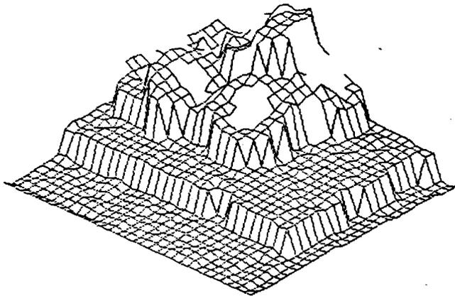
A pair of images are obtained under the random texture illumination using a pair of vidicon TV cameras for the PRISM stereo system. A pair of brightness arrays for the binocular PRISM stereo are shown in Fig. 5. The output of the PRISM stereo as a perspective plot are shown in Fig. 6.
