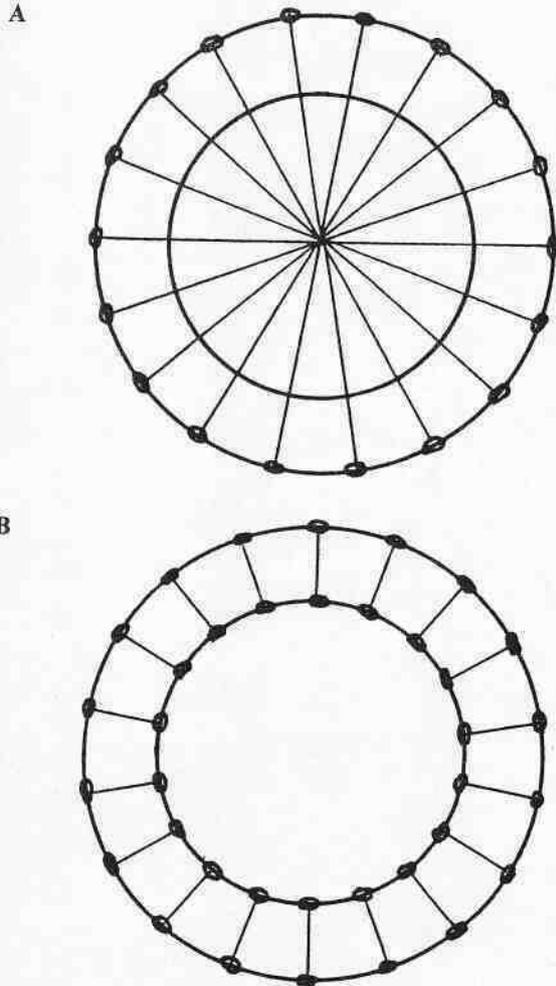
Fig. 18. The legal grasp configurations and the world coordinate. The gripper approach direction,  $(-a, -b, -c)$  is  $(-D_x, -D_y, -D_z)$  where  $(D_x, D_y, D_z)$  is a normal vector perpendicular to the plane, the gripper normal direction is the direction from the grasp point to the center of the 2D ring specified by  $\alpha$ .
