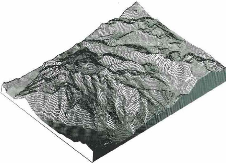
Figure 10: "Block-diagram" representation of terrain surface. This is an isometric projection of a series of uniformly spaced vertical profiles of the surface viewed from the south-east. Note the shading effect due to the variation in line spacing.
