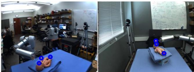
Figure 7. The Camshift tracker is used to track the robot end-effector as well as two points on the line in the workspace.
