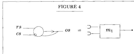
It should be noted that this  $\boxed{m_1}$  corresponds to the actual vacuum tube trigger circuits mentioned at the beginning of 5.1. It is worth mentioning that  $\boxed{m_1}$  contains one E-element, while the simplest trigger circuits contain one or two vacuum tubes (cf. loc. cit.), in agreement with the estimates of 6.5.
