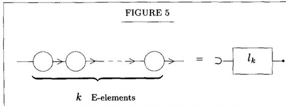
and provide it with such terminal equipment (at both ends, possibly connecting them) as may be required in each particular case. This simple line is shown again in Figure 5. Terminal equipment, which will normally cycle the output  $os$  at  $\boxed{l_k}$ 's right end back into the input at its left end, but upon stimulation at  $s$  suppress (clear) this returning of the output  $os$  and connect instead the input with the line  $rs$ , is shown in Figure 6.
