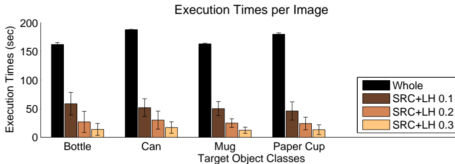
Fig. 10: Average execution times of each strategy. Our SRC+LH strategies outperform the whole detection strategy in computing times. The error bars represent the standard deviation of execution times.
