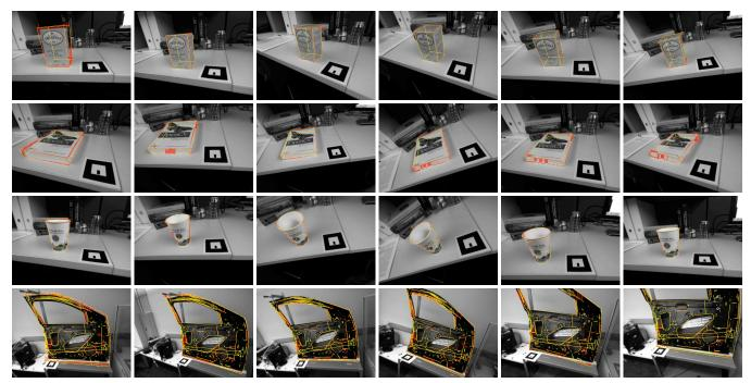
Fig. 6: Tracking results of the four targeted objects. From top to bottom, teabox, book, cup and car door. From left to right, t < 10, t = 100, t = 200, t = 300, t = 400 and t = 500 where t is the frame number. The very left images are results of the GPE.
