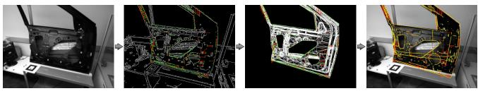
Fig. 4: The flow of the LPE. From the input image, an edge image is obtained using the Canny edge detector, and the CAD model is rendered with the prior pose. After calculate the error between the projected model and edge image, Iterative Re-weighted Least Square estimates the posterior pose. The estimated pose is shown in the last image.
