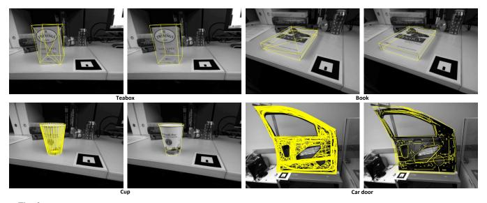
Fig. 3: Original and simplified CAD models. By using the salient edges selection, we can get a set of good model edges to track.
