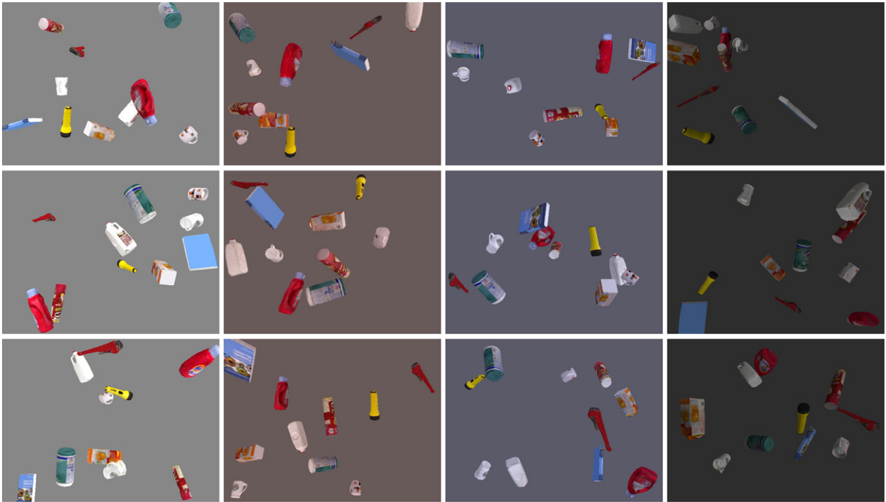
Fig. 20. Example images of the color quantization step learning dataset. The dataset consists of 50 scenes, where object mesh models are rendered with random poses, and ground truth poses. To find a robust quantization step to illumination variations, four different lighting conditions are considered: normal, red, blue, and dark lights. (For interpretation of the references to color in this figure, the reader is referred to the web version of this article.)
