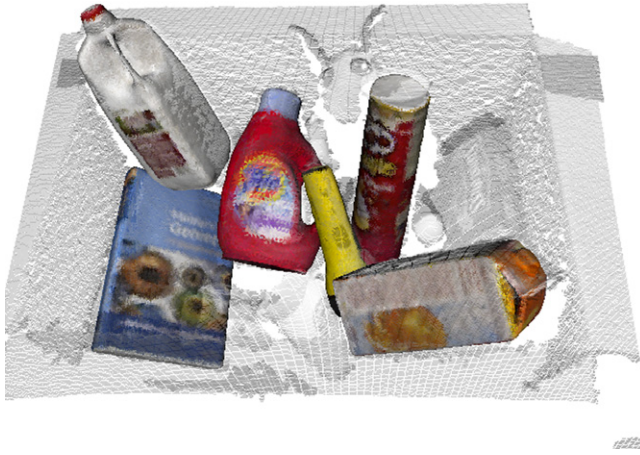
Fig. 1. Overview. Our approach exploits both geometric shape and photometric color information in point clouds for robust object pose estimation. The estimated pose of each object is depicted as a color mesh model. Since our approach does not hinge upon the planar segmentation, it can be applied in highly cluttered environments wherein the planar segmentation might not be applicable.
