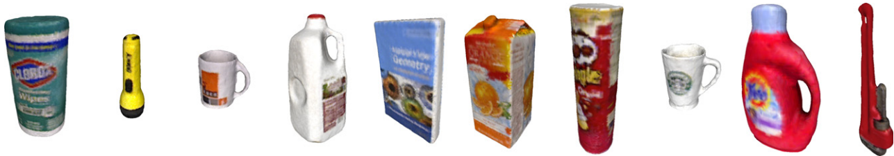
Fig. 6. Polygonal mesh models of the test objects. Ten daily objects were chosen. Each object model is obtained by combining multiple views of object point clouds, followed by the Poisson reconstruction algorithm [56]. From left to right: Clorox , Flash , Kuka Mug , Milk , MVG Book , Orange Juice , Pringles , Starbucks Mug , Tide , and Wrench .
