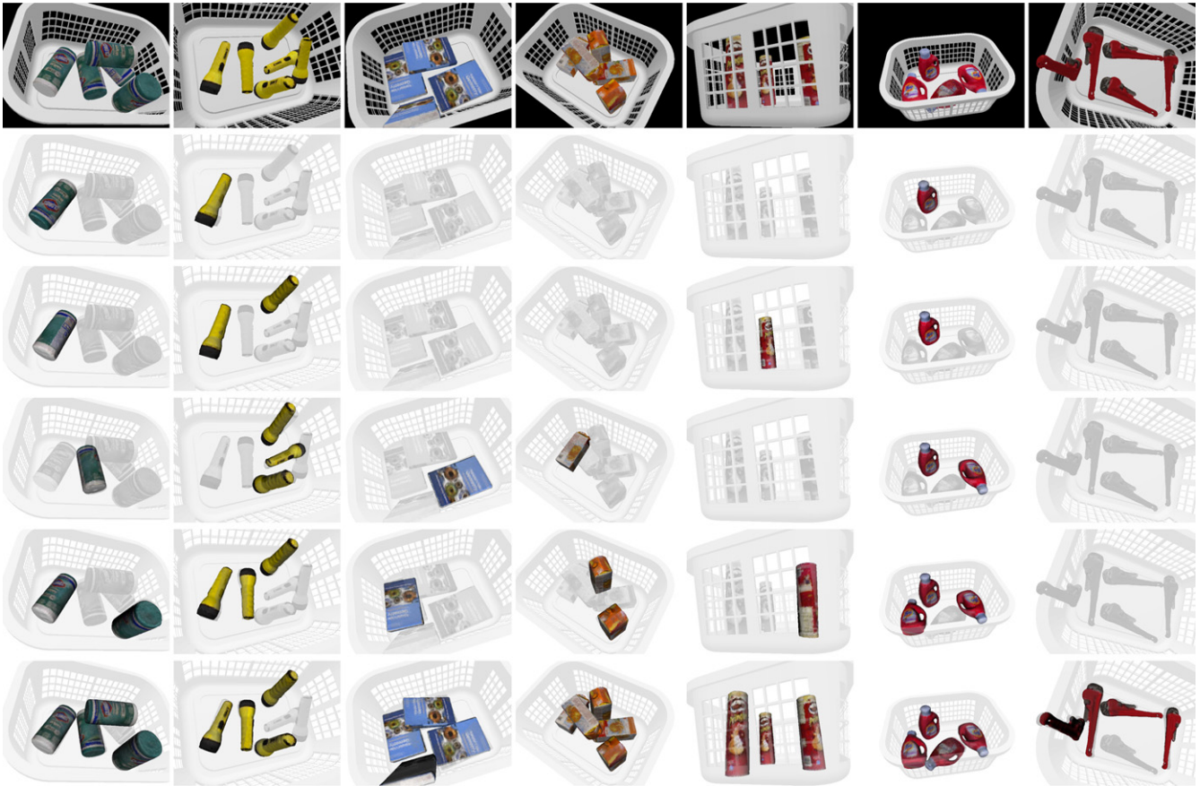
Fig. 14. Selected pose estimation results of Hinterstoisser et al. [16] without the ICP (second row), Hinterstoisser et al. [16] with the ICP (third row), Papazov et al. [48] (fourth row), Drost et al. [33] (fifth row), and our approach (sixth row) in the SOMI dataset. Our approach can handle the multiple instances scenario well, whereas Hinterstoisser et al. [16] and Papazov et al. [48] fail to recognize multiple instances in most cases.
