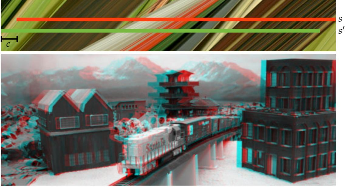
**Figure 6.4:** A 2D EPI of a light field, showing two planar  $uv$ -cuts. The horizontal offset  $c$  changes the convergence plane of the stereoscopic image pair. The bottom image shows the corresponding stereoscopic image pair generated from  $I_s$  and  $I_{s'}$ .
