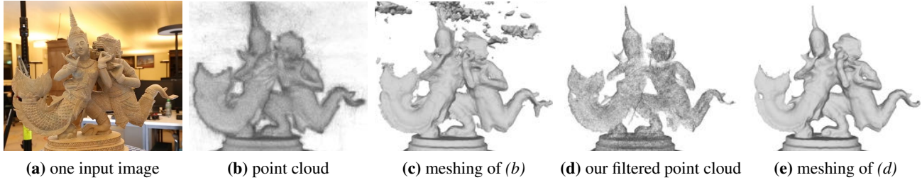
Figure 1. From a set of images of a scene (a), multi-view stereo methods such as [9] can reconstruct a dense 3D point cloud (b), which however often suffers from noise and outliers. This leads to disturbing artifacts when used in subsequent surface reconstruction (meshing) methods such as [20] (c). We propose a simple and efficient filtering method that produces clean point clouds (d) that allow for a favorable surface reconstruction (e).
