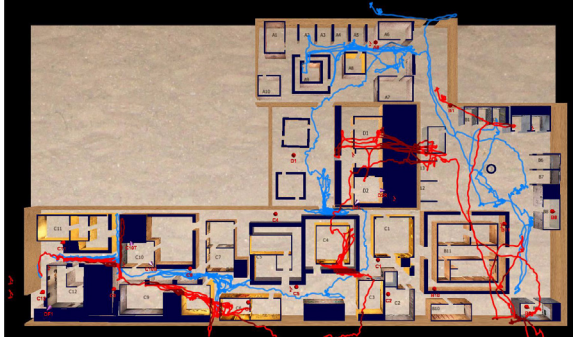
Figure 10. The comparison between the estimated trajectories with continuous landmark correction or not.
