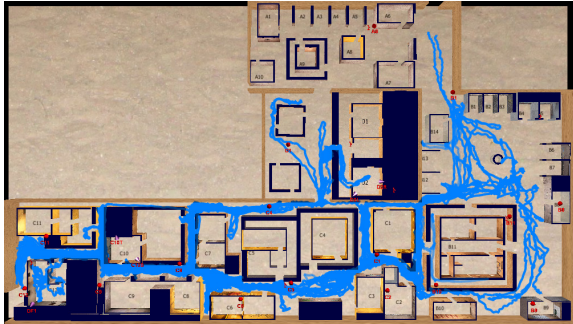
Figure 11. The bird view of the estimated 3D trajectories overlaid in the IIT 3d model.
