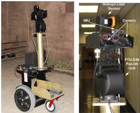
Figure 1. A segway robotic platform (RMP400) with LIDAR-camera sensor unit.
