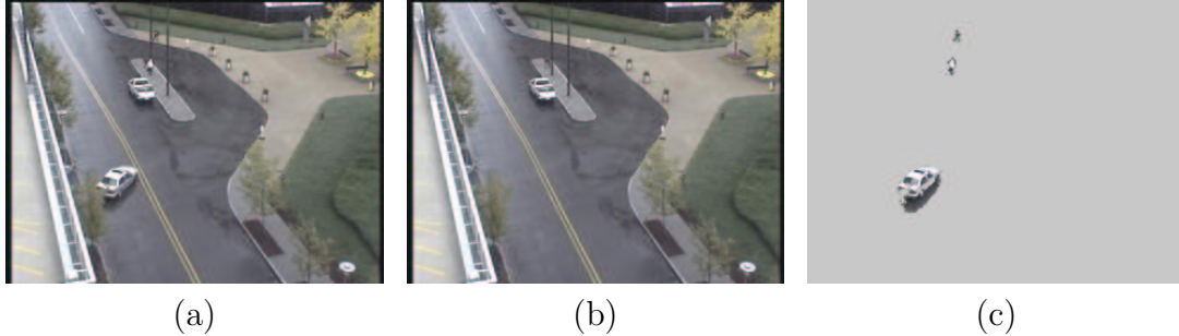
Figure 3-1: An illustration of background subtraction: (a) a video frame, (b) current background model, and (c) pixels identified as belonging to the foreground (shown against a light-grey background for clarity). Note the parked car in (b), which is considered part of the background, and the shadow of the moving car in (c), which is detected as foreground.
