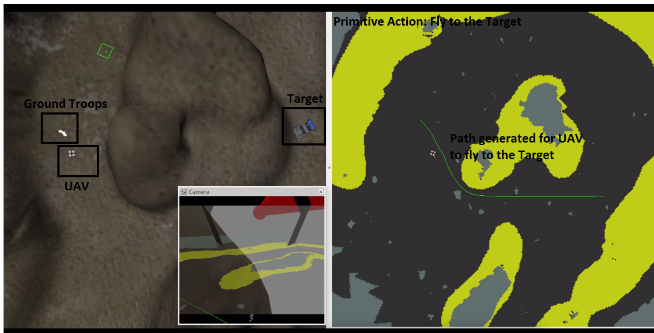
Figure 7. Now the UAV has updated its belief of where it thinks the target is located, and it must go increase this belief further by directly observing the target. The green path shown on the right is the path it generates and follows to reach the target.
