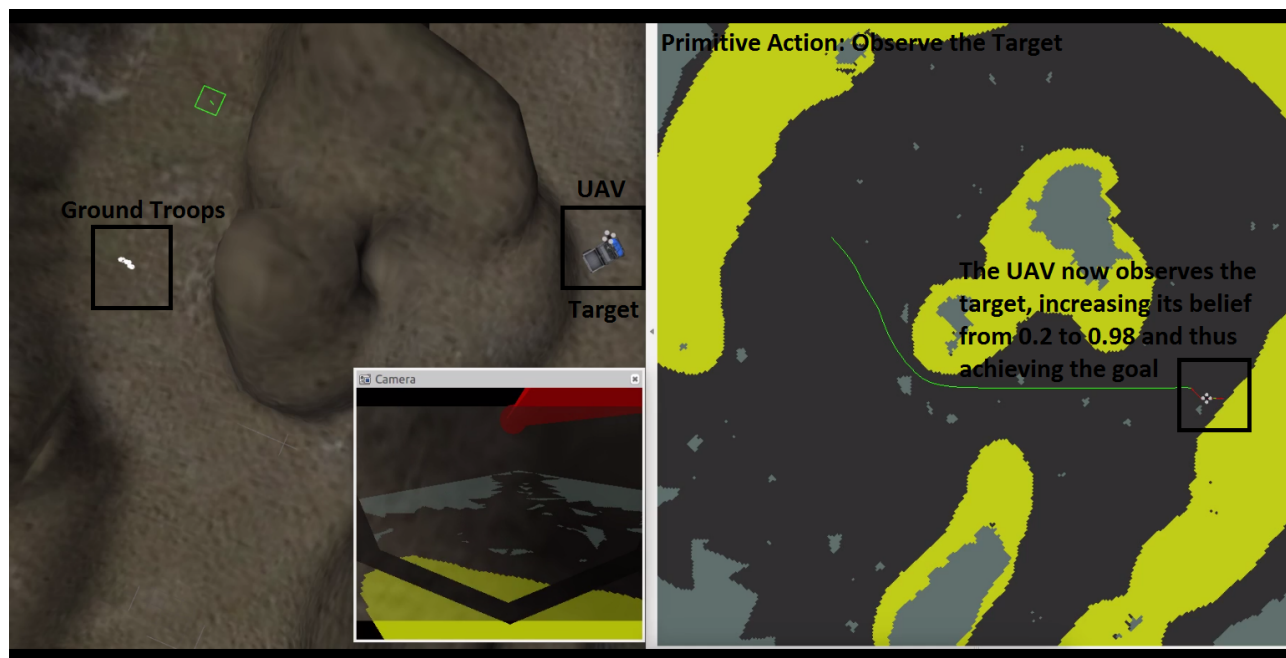
Figure 8. Finally, the UAV observes the target several times to verify that it is in the believed location. The reason so many observations are made (as you can see in Figure 3) is due to the noise in the sensor.
