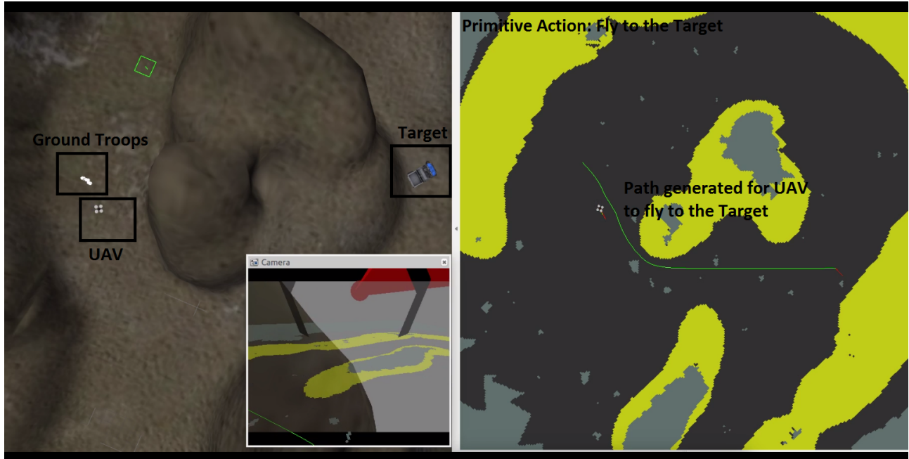
Figure 10: Now the UAV has updated its belief of where it thinks the target is located, and it must go increase this belief further by directly observing the target. The green path shown on the right is the path it generates and follows to reach the target.
