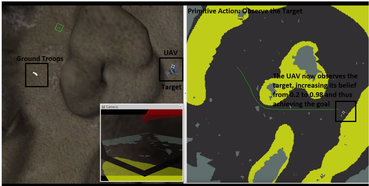
Figure 11: Finally, the UAV observes the target several times to verify that it is in the believed location. The reason so many observations are made (as you can see in Figure 7) is due to the noise in the sensor.
