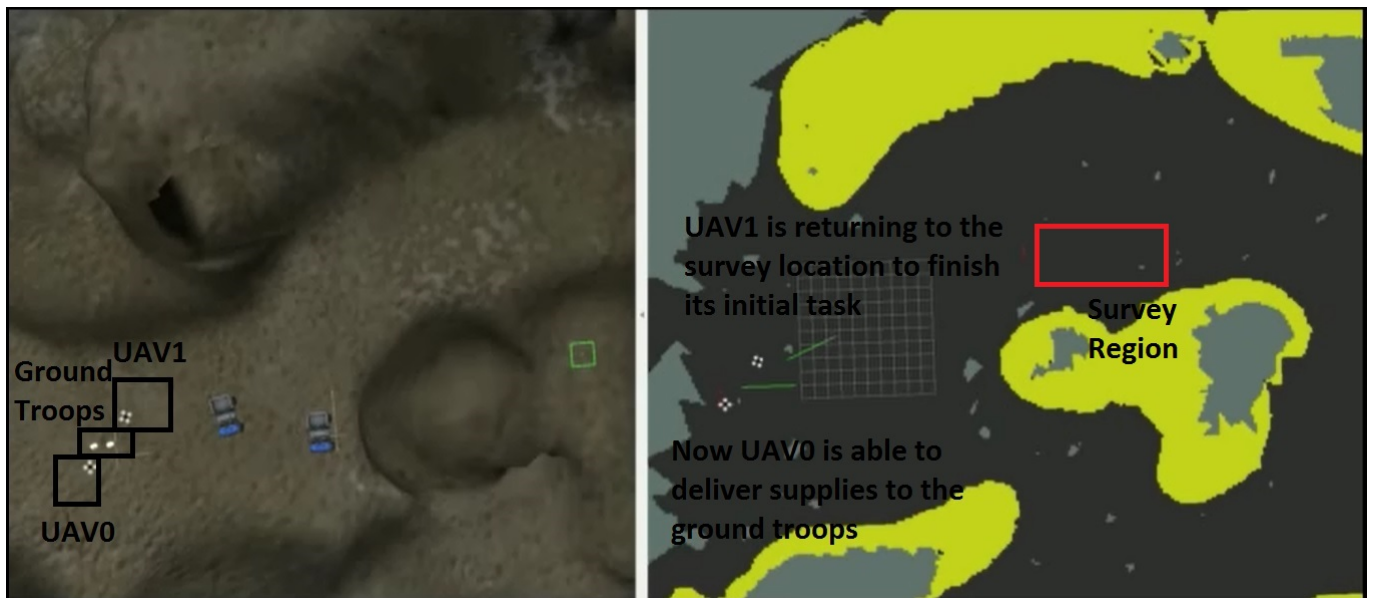
Figure 15: UAV0 is in transit to the ground troops now that it knows their location. Once it arrives, it delivers the necessary supplies. UAV1 has returned to its original objective, and is in transit of the survey region.
