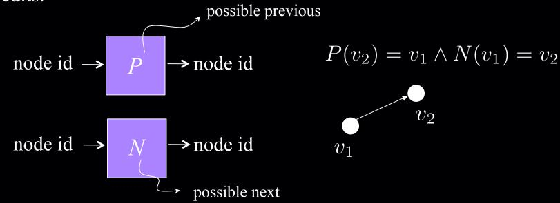
**END OF THE LINE**: Given P and N: If  $0^n$  is an unbalanced node, find another unbalanced node. Otherwise say "yes".
