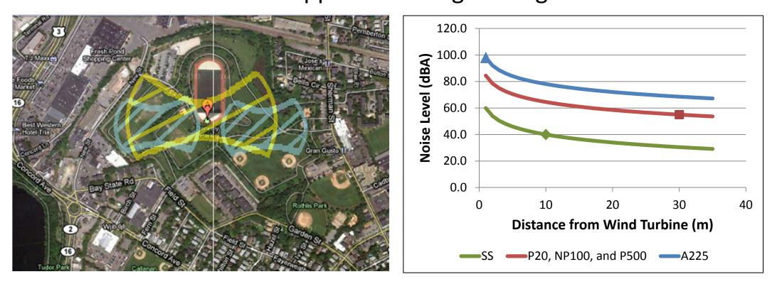
Another community impact issue associated with wind turbine development is noise level. Each turbine has a noise (sound pressure) level that decreases as a function of distance from the turbine, as shown in the above graph.
