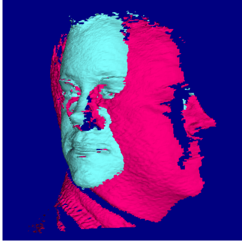
Figure 5.3: Snapshot of the FacesPat1_000U01-144U01_N_0003 test. Demonstrates a catastrophic failure of the registration when large non-overlapping regions exist and no corresponding point pairs are classified as outliers
