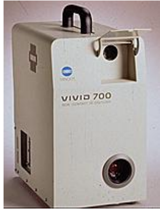
Figure 5.2: Photo of the Minolta Vivid 700 Range Sensor [1]
