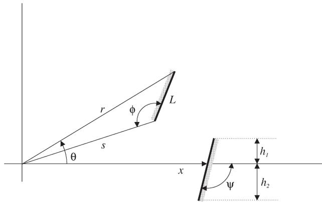
Fig. 27. Library entry F-2: an implementation for curve F (“cam and centered follower”). The two faces are shown as thick lines. The rotating face rotates about the origin; the translating face translates horizontally.  $\theta$ , measured positive counterclockwise, is the angle of the rotor;  $x$ , measured positive to the *left*, is the position of the slider.
