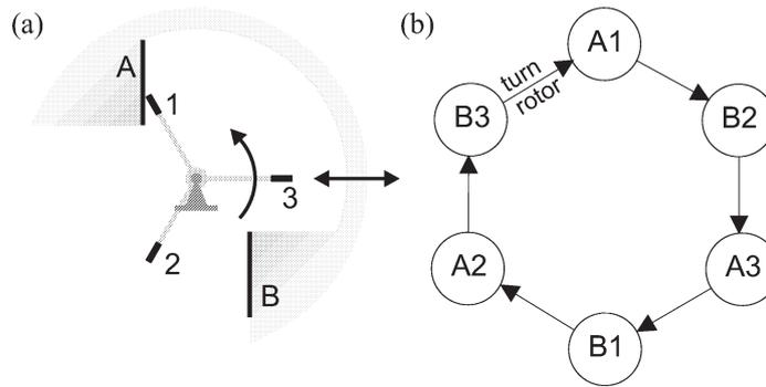
Fig. 39. (a) The stylized sketch of the yoke and rotor device. (b) The desired behavior. The letter and number in each node indicate which yoke face and which rotor face are engaged in that state. Turning the rotor is the external input that causes each of the transitions.
