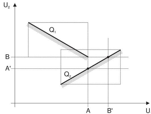
Fig. 24. Two non-intersecting, finite qcs-curves with intersecting bounding boxes.
