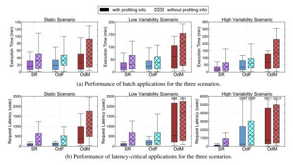
Figure 4: Performance of jobs of the three workload scenarios with the three provisioning strategies. The boundaries of the boxplots depict the 25th and 75th percentiles, the whiskers the 5th and 95th percentiles and the horizontal line in each boxplot shows the mean.
