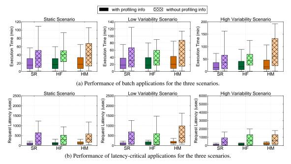
Figure 10: Performance of the three scenarios with the statically-reserved and hybrid provisioning strategies. The boundaries of the boxplots depict the 25th and 75th percentiles, the whiskers the 5th and 95th percentiles and the horizontal line in each boxplot shows the mean.
