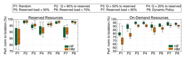
Figure 6: Sensitivity to the policy of mapping jobs to reserved versus on-demand resources for HF and HM.
