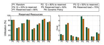
Figure 7: Utilization of reserved resources and cost with different application mapping policies for HF and HM.
