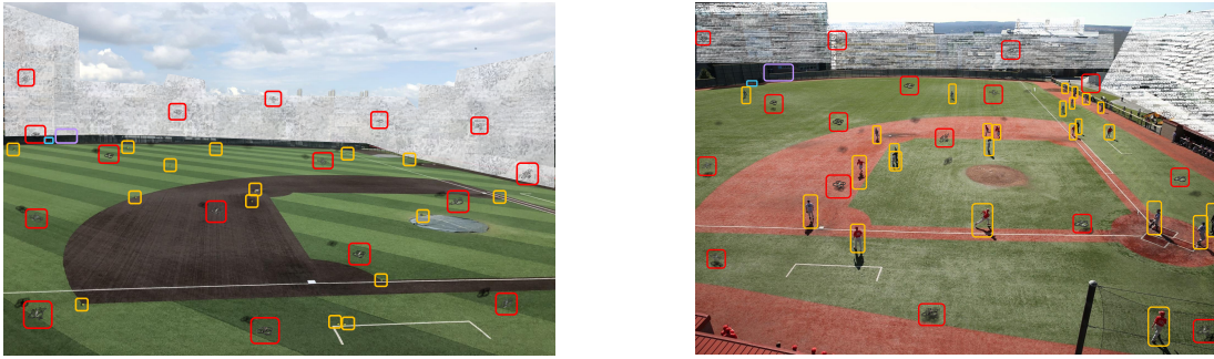
Figure 2: The drone swarm executing (a) the first scenario where the number and location of a set of static items (tennis balls) is determined, and (b) the second scenario, where the number of unique people in a field is determined.
