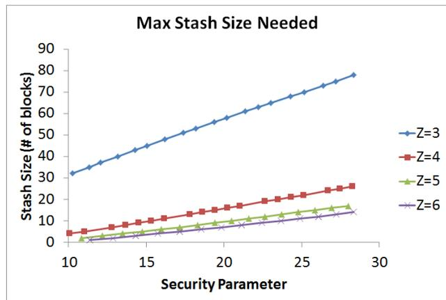
**Figure 2: Empirical estimation of the required stash size to achieve failure probability less than  $2^{-\lambda}$  where  $\lambda$  is the security parameter. Measured for  $N = 2^{16}$ , but as Figure 3 shows, the stash size does not depend on  $N$  (at least for  $Z = 4$ ). The measurements represent a worst-case (in terms of stash size) access pattern. The stash size does not include the temporarily fetched path during Access.**
