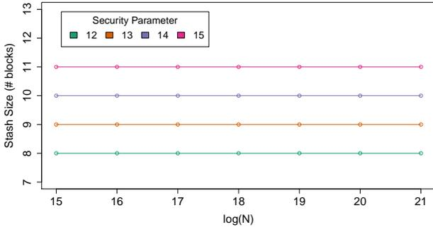
Figure 3: The stash size to achieve failure probability less than  $2^{-\lambda}$  does not depend on  $N$  ( $Z = 4$ ). Measured for a worst-case (in terms of stash size) access pattern. The stash size does not include the temporarily fetched path during Access.
