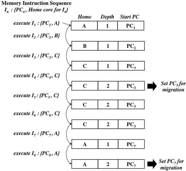
Fig. 2. An example how instructions (or PC's) which are followed by consecutive accesses to the same home location, i.e., *migratory instructions* are detected in the case of the depth threshold  $\theta = 2$ . Setting  $\theta = 2$  means that a thread will perform remote accesses for “one-off” accesses and will migrate for multiple accesses ( $\geq 2$ ) to the same home core.
