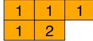
Figure 6. Macroblock dependence in image processing section of H.264. A macroblock is dependent on neighboring macroblocks above-left, above, above-right, and to the left. All macroblocks labeled “1” must be processed before the macroblock labeled “2.”
