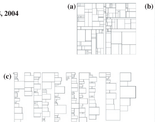
Figure 3. A space-filling layout (a) saves space but does not convey time; a timeline (b) wastes space and requires excessive panning due to severe aspect ratio; weaving the timeline along both dimensions (c) conveys time and achieves reasonable aspect ratio.
