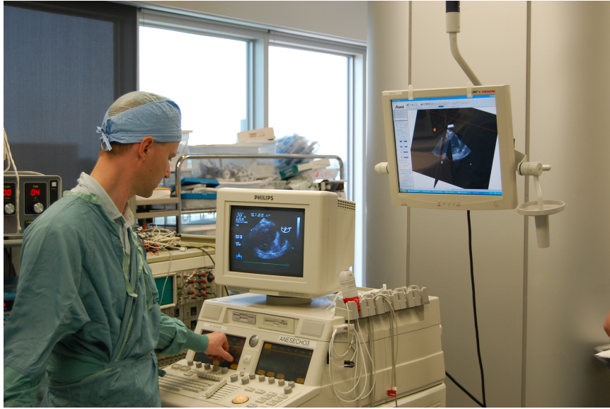
Fig. 2.4: Real-time 4D ultrasound reconstruction in progress. A monitor positioned close to the clinician visualizes the AtamaiViewer output, which shows the partially reconstructed output volumes being filled in in as the clinician manipulates the ultrasound probe.
