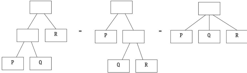
Fig. 17: Transformations based on the identity  $(P; Q); R = P; (Q; R) = P; Q; R$
