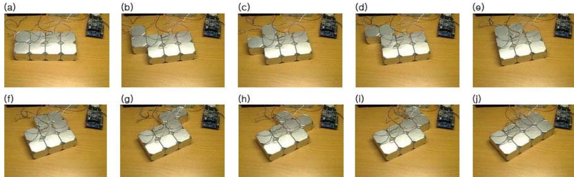
Fig. 16. EM-Cube surface locomotion experiment on sheet Polyvinylchloride
