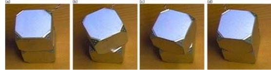
Fig. 6. Sequence of EM-Cube Spinning
